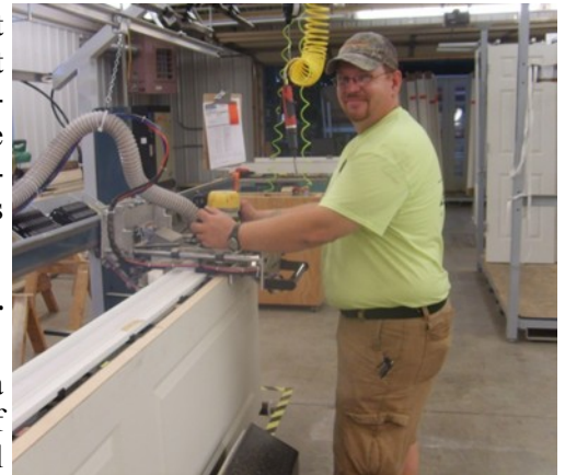
Joe Andrews machines a new door for lock, hinges and jambs.
